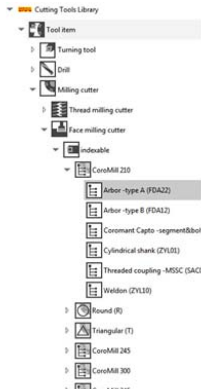
Example of branches in the GTC structure.
